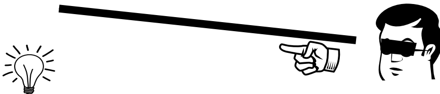
FIGURE 2-4 The open-loop control error is large with eyes closed.
