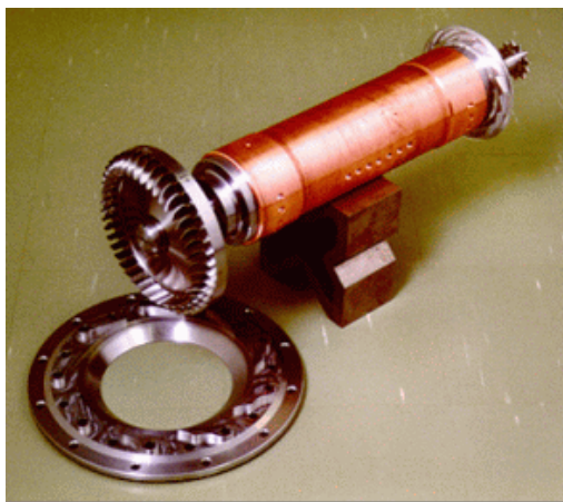
Left: The turbo generator main parts, the super sonic turbine in front. Right: The ORC power plant in tests in LUT.
