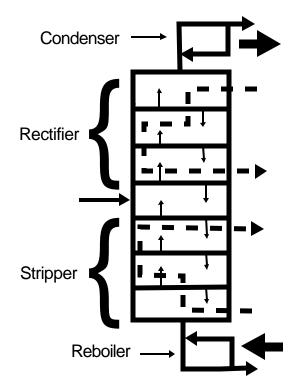
Figure 2: Conventional column retrofitted with serial heat exchangers.
