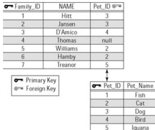
Figure 2-5: Example of a NULL value for a foreign key
