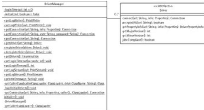
Figure 4–7: UML class diagram of Driver and DriverManager
