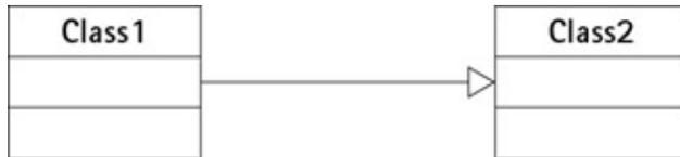
Figure D–8: Generalization and inheritance example
