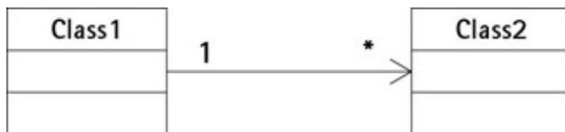
Figure D-7: One-to-many-multiplicity diagram
