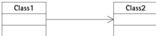
Figure D-5: Unidirectional-association example
