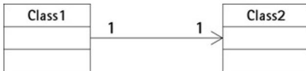
Figure D-6: One-to-one-multiplicity diagram
