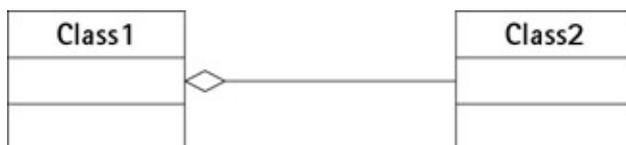
Figure D–11: Aggregation example
