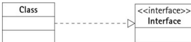
Figure D–9: Realization example
