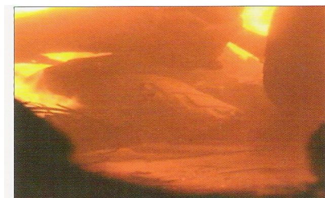
Internal view of the HOTDISC during operation with whole tires
