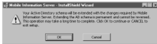
Figure 7.3 MIS Extends the Active Directory Schema and Adds a Microsoft Mobility Admins Group
