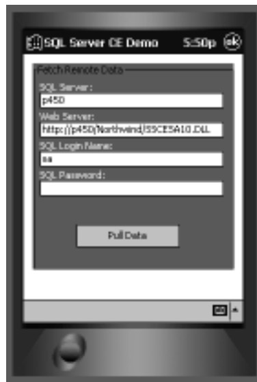
Figure 7.55 At the Login Screen, the Pocket PC Pulls Data from the SQL Server Using IIS
