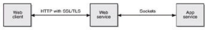
Figure 10-2: A scenario using SSL or TLS to protect client and server data.
