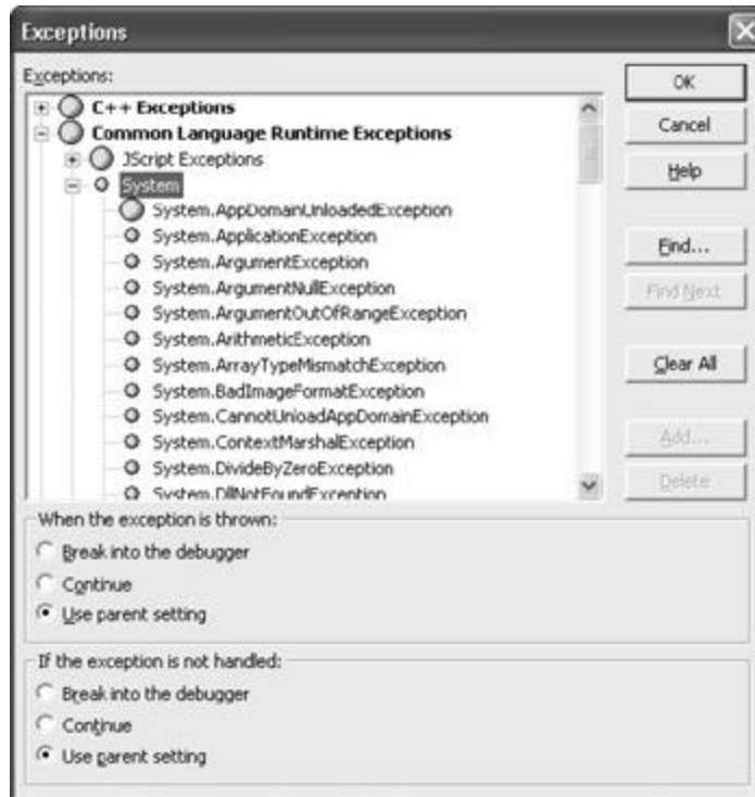
Figure 18-6 : Visual Studio .NET Exceptions dialog box showing CLR exceptions defined in the System namespace
