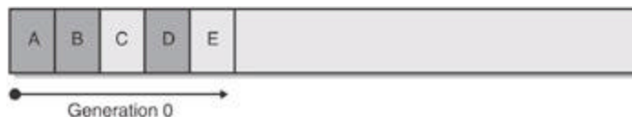
Figure 19-7 : A newly initialized heap containing some objects; all in generation 0. No collections have occurred yet.
