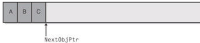
Figure 19-1 : Newly initialized managed heap with three objects constructed in it
