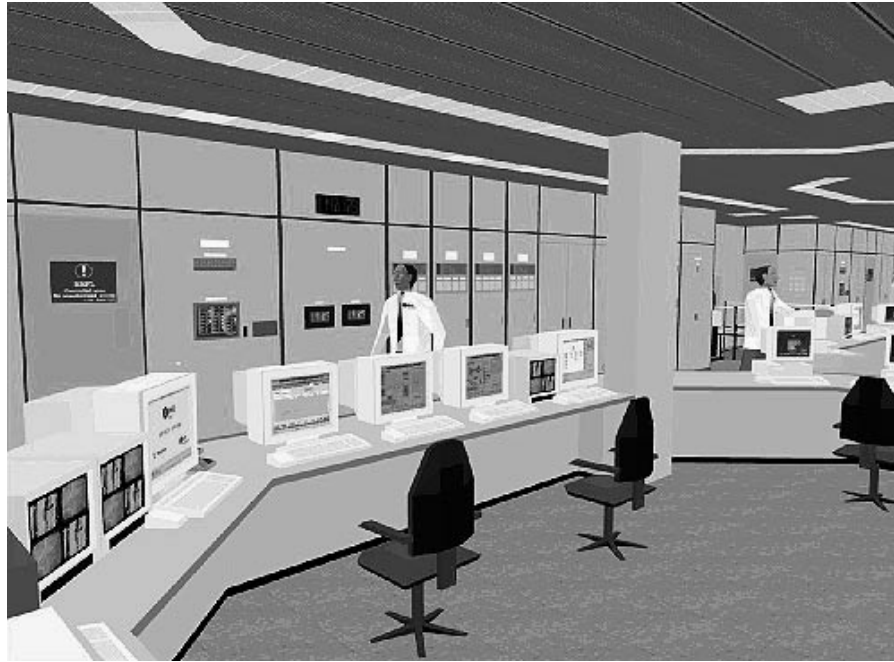
Figure 8.2. Virtual nuclear facility central control room for ergonomics assessment and operational training.
