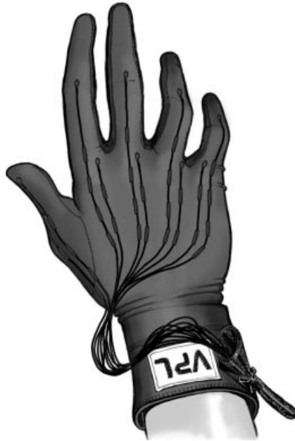
Figure 1.2. The WristSystem, based on the VR DataGlove.
