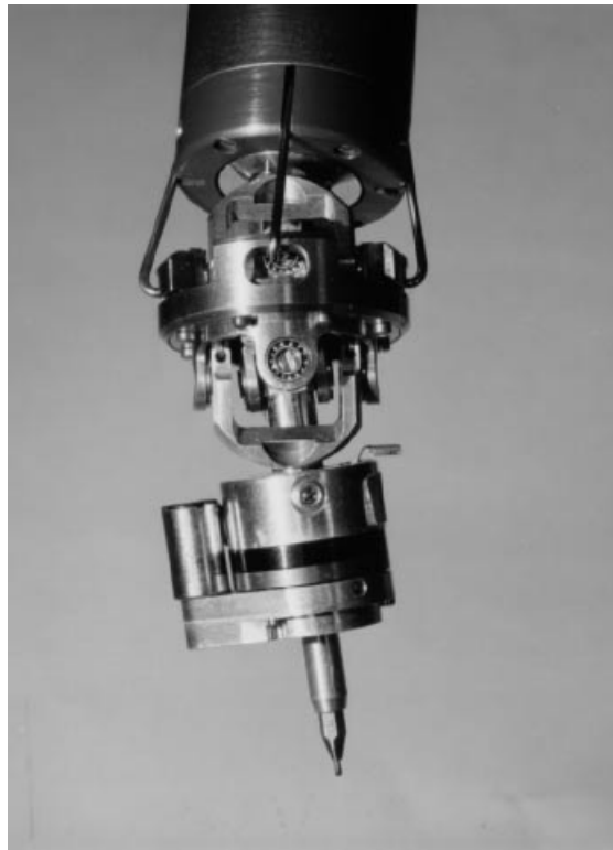
Figure 4.6. Slave robot end effector with force sensor and microforceps.
