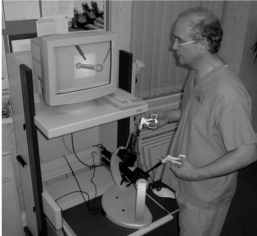
Figure 8.6a. The Latest Version of MISTVR, Showing Re-Engineered Instruments and One of Three New Gynaecological Tasks.
