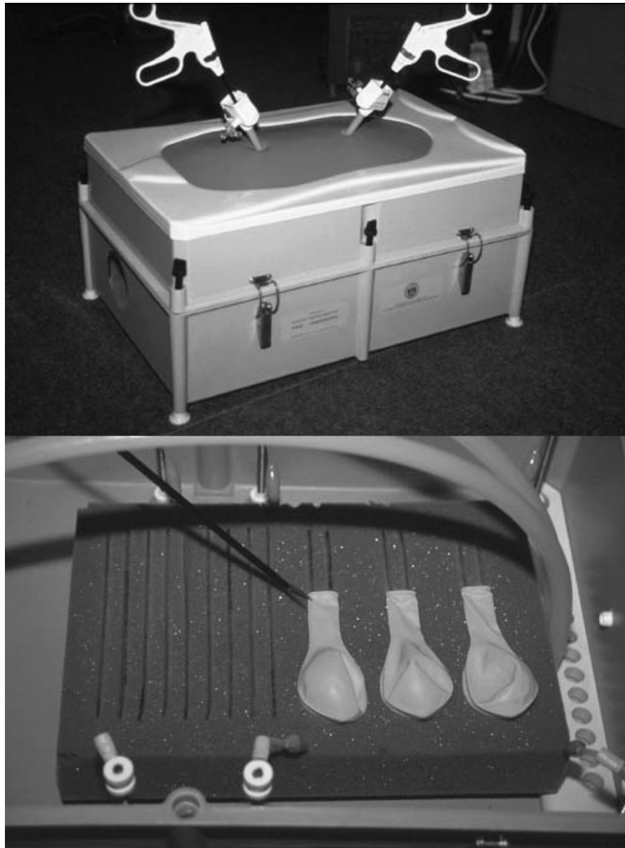
Figure 8.6b. A Conventional Physical Closed Box Endoscopic Trainer, Showing Synthetic Contents.
