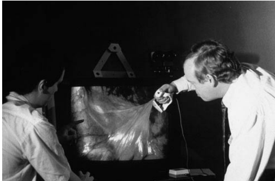
Figure 8.5. Early British deformable tissue simulation using Logitech Ultrasonic Space Tracker prototype.
