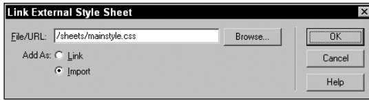
Figure 20-3: Use the Link method for style sheets readable by older browsers like Netscape 4.x.
