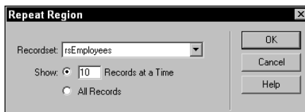
Figure 17-2: With the Repeat Region server behavior, you can show some or all of the records in the chosen recordset.
