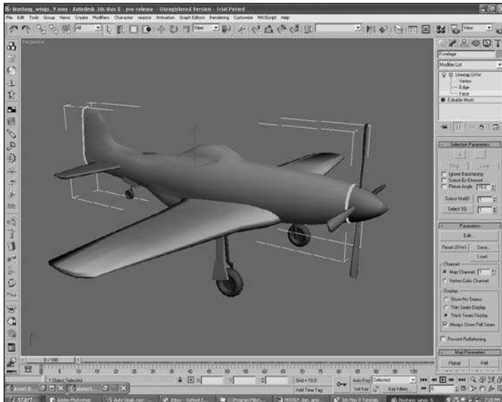
Figure 4.72 Use the Unwrap UVW modifier and select the faces.
