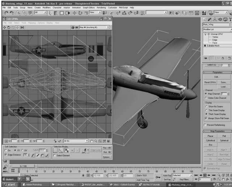
Figure 4.79 UVWs are assigned to the top half of the main wing in the Edit UVWs window.
