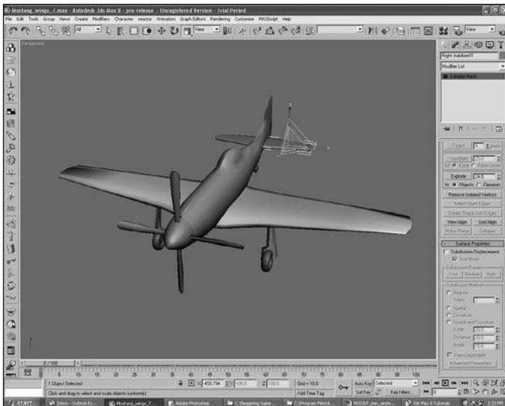
Figure 4.59 The rear elevator, main wheels, main gear doors, and rear landing gears are in position.
