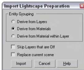
Figure 3-10: The Import Lightscape Preparation dialog box can specify how entity grouping is derived.
