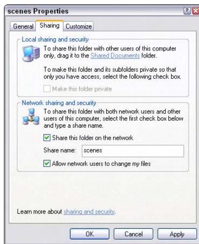
Figure 45-3: Sharing a directory so that other computers on the network can use it
