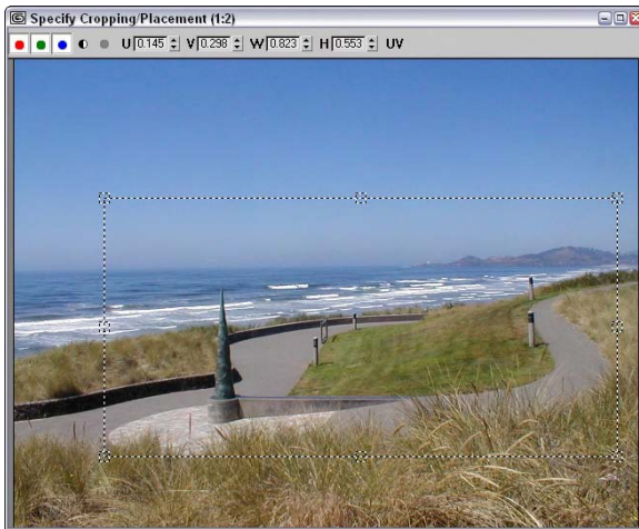
Figure 22-8: Viewing an image in the Cropping/Placement dialog box enables you to set the crop marks.
