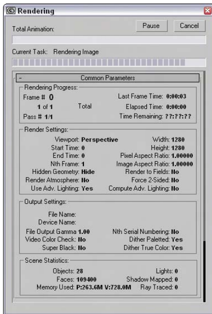
Figure 41-5: The Rendering dialog box displays the current render settings and progress of the render job.
