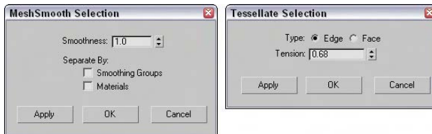
Figure 14-13: The Settings dialog boxes for the MSmooth and Tessellate buttons let you interactively set the Smoothness and Tension values.
