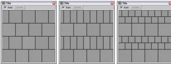
Figure 22-14: From the Standard Controls rollout, you can select from several preset Tile styles, including Running Bond, English Bond, and Fine Running Bond.
