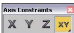
Figure 10-6: The Axis Constraints toolbar includes buttons for restricting transformations to a single axis or plane.
