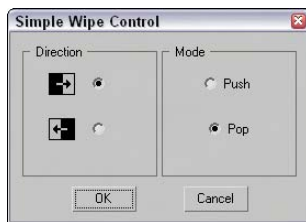
Figure 47-7: The Simple Wipe Control dialog box lets you select which direction to wipe the image.
