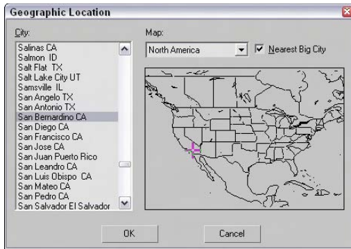
Figure 27-13: The Geographic Location dialog box lets you specify where you want to use the Sunlight system. You have many different cities to choose from.
