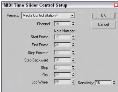
Figure 4-25: The MIDI Time Slider Control Setup dialog box lets you set up specific notes to start, stop, and step through an animation.
