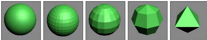
Figure 5-10: Sphere primitives of various Segment values with the Smooth option turned on and off
