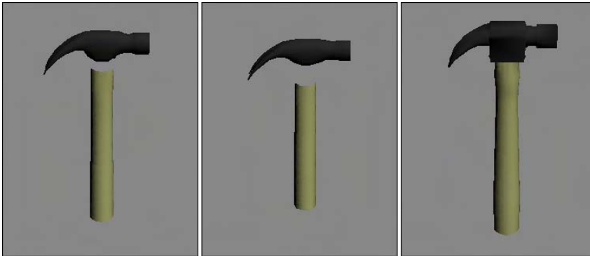
Figure 11-20: The Relax modifier can simplify the number of vertices in an object.
