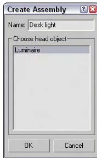
Figure 8-2: The Create Assembly dialog box lets you choose a light head object.
